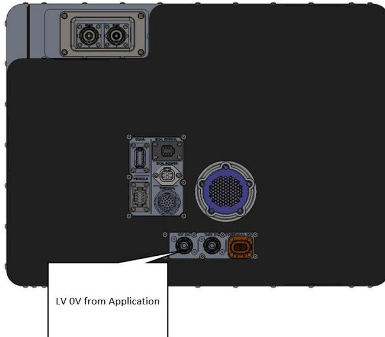
Figure 23: Location of 0V LV connector on FCM.
