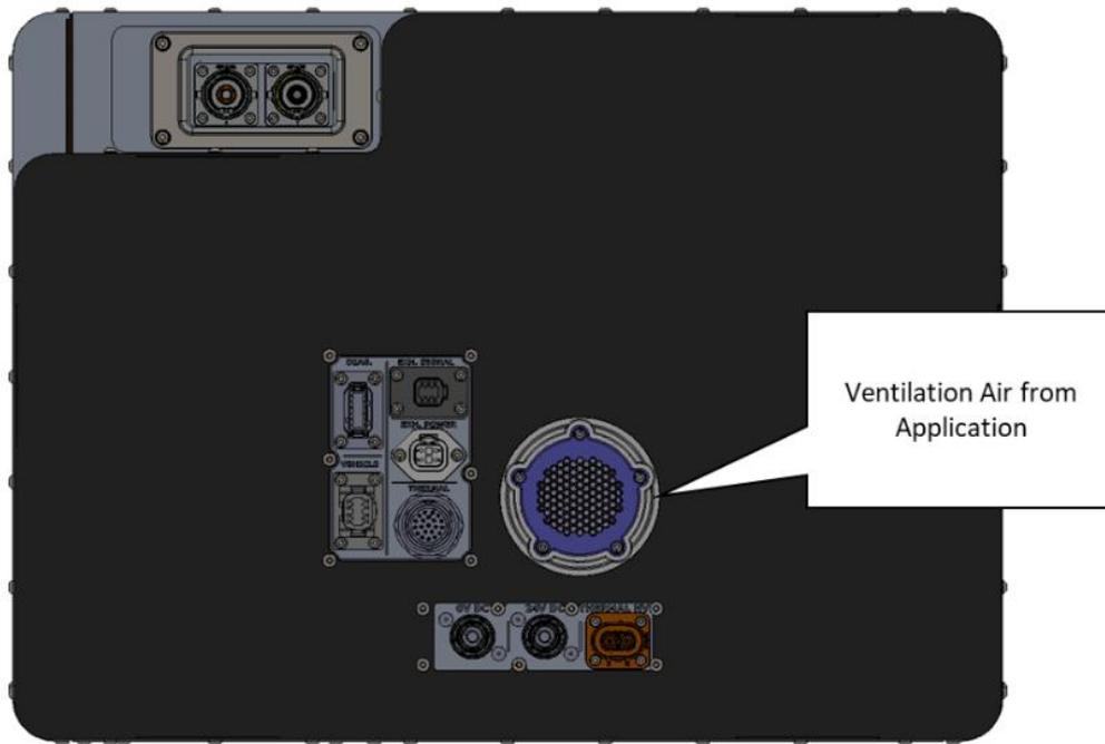
Figure 21: Ventilation air inlet location identified.
