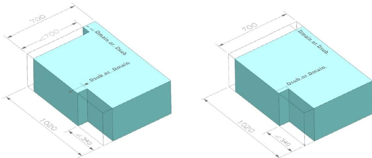
Figure 5: Example of FC module interface area with 1<sup>st</sup> side and optional 2<sup>nd</sup> side
