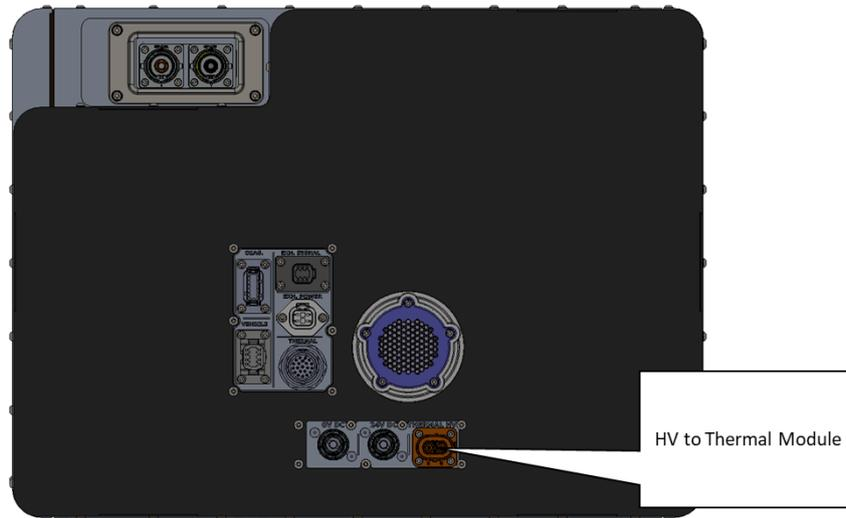
Figure 28: Location of HV to Thermal Module DCDC connector on FCM.
