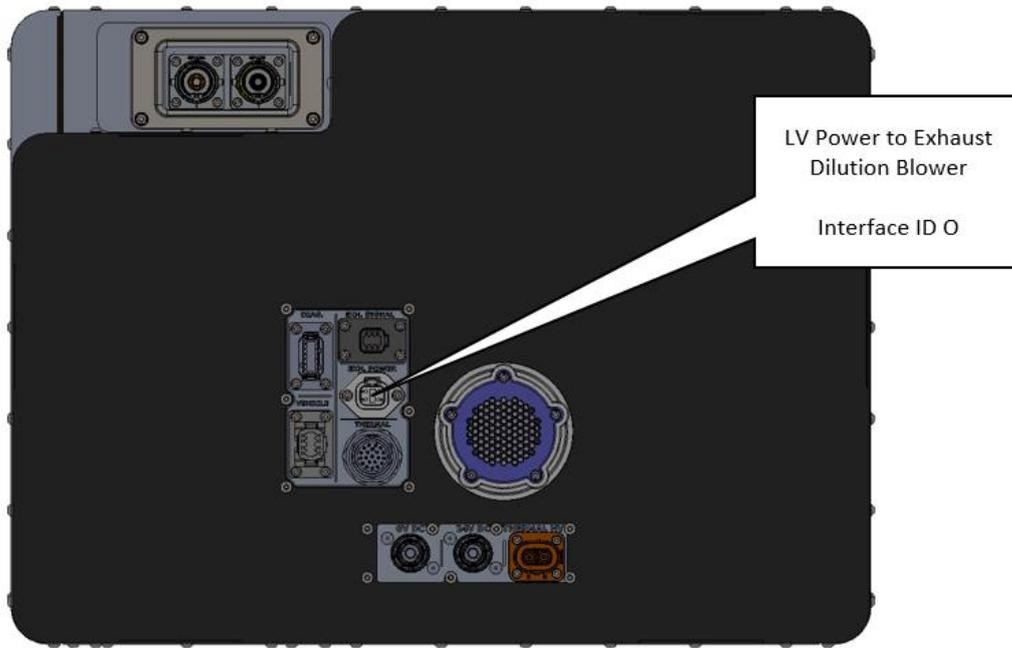
Figure 26: Location of exhaust module LV connector on FCM.
