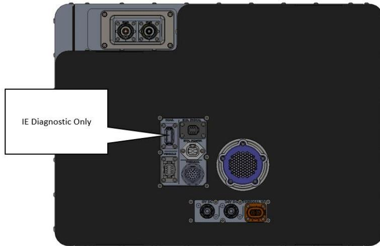
Figure 30: Location of IE Diagnostic connector on FCM.
