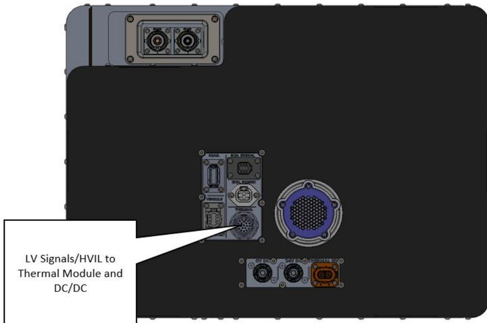
Figure 24: Location of Thermal module LV connector on FCM.
