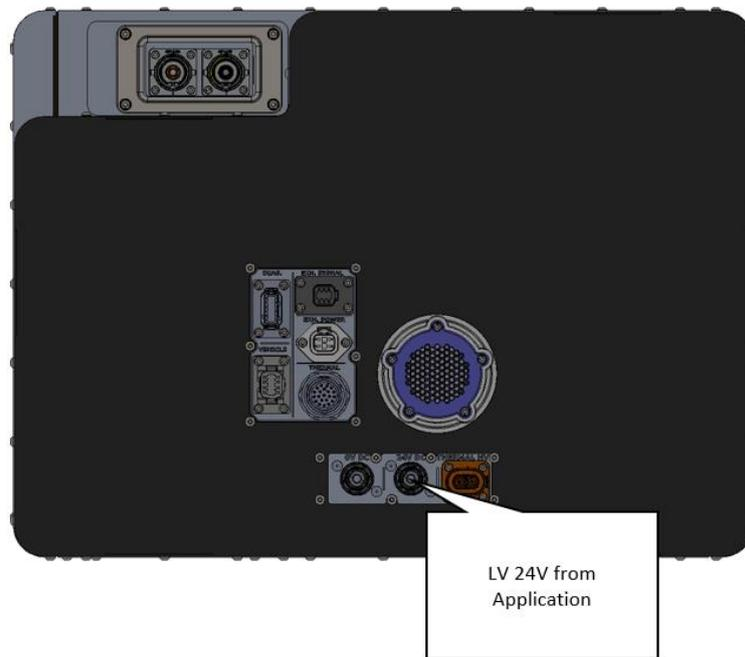
Figure 22: Location of 24V LV connector on FCM.
