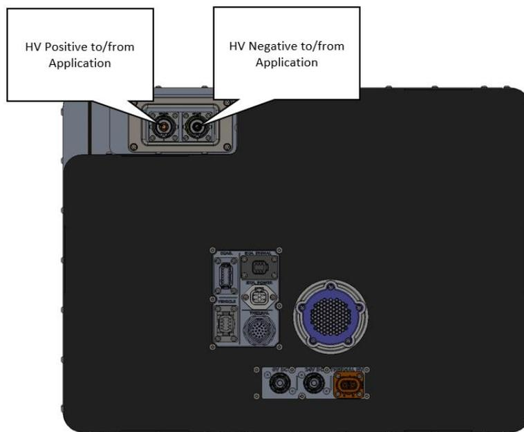
Figure 27: Location of HV to/from application connector on FCM.
