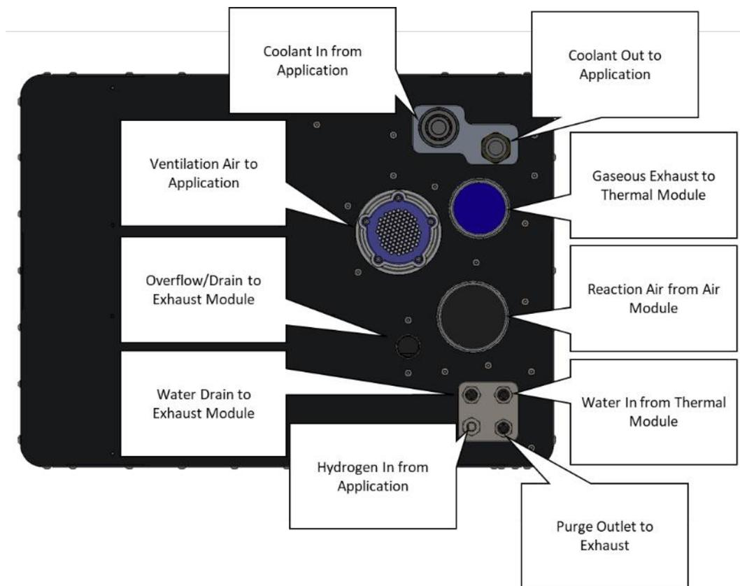
Figure 20: FCM hydraulic and pneumatic connections identified.
